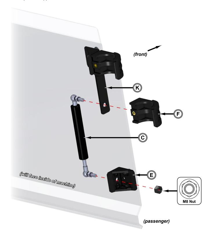
Install Upper Windshield (A) to Roll Cage with bolts included with Clamps (F).
