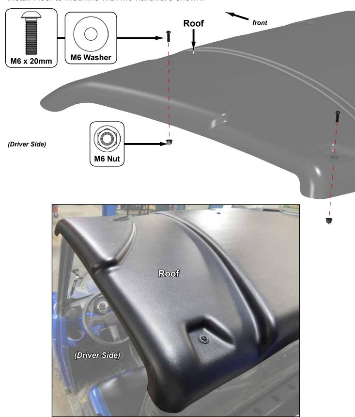
Align Roof to machine and tighten hardware completely
